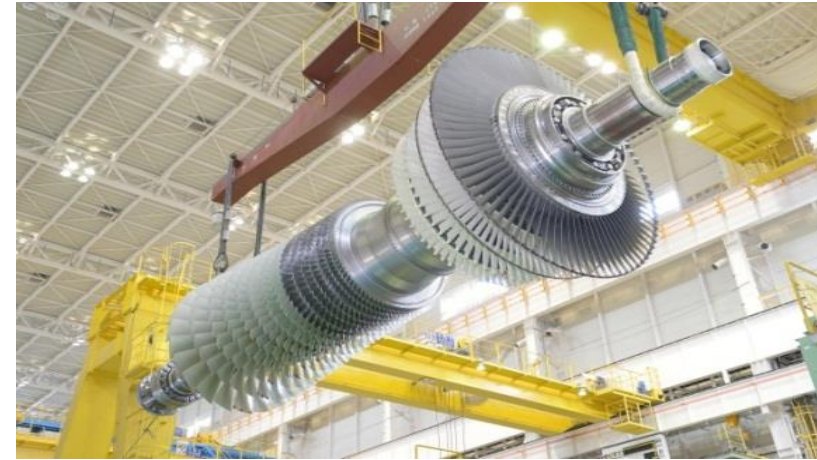
Large frame gas turbine
